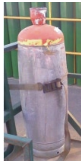
Cylinder bulging and paintwork flaking (immersion?)
