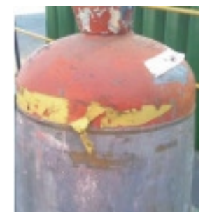
Cylinder bulging and paintwork flaking (immersion?)
